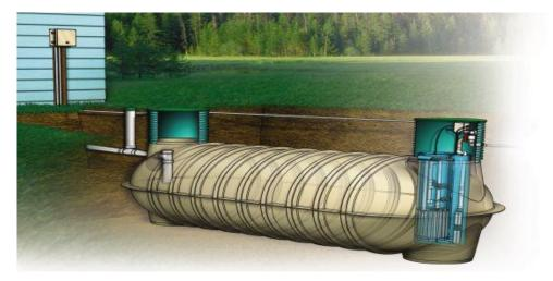
The STEP system comprises of a septic tank with a pump. It pre-treats wastewater. This is then pumped to a central piping network and on to the treatment plant. The STEP system is thus an alternative to grinder pumps or Biolytix units connecting houses to a central piping system. In all cases, outflow is highly treated at the treatment plant before it is released on to land.
