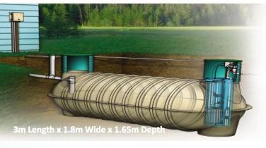
The STEP system comprises of a septic tank with a pump. It pre-treats wastewater. This is then pumped to a central piping network and on to the treatment plant. The outflow is highly treated at the treatment plant before it is released on to land.
