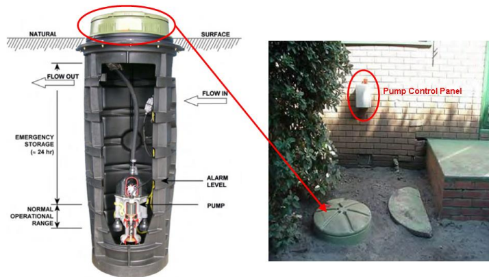
Figure 2. Low Pressure Grinder Pump System, Rotorua Lakes Council, Sewerage Options for Tarawera, Manzano 2017
