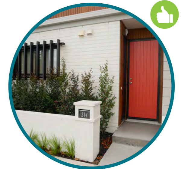
Terraced House, Hobsonville. Clearly visible door, low height fencing and landscaping contribute to an attractive frontage.
