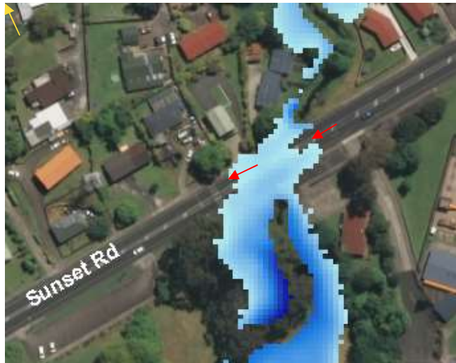
Figure 5-25 Flood depths (model prediction), Sunset Road, Otamatea Stream (upstream culvert), August 2014
