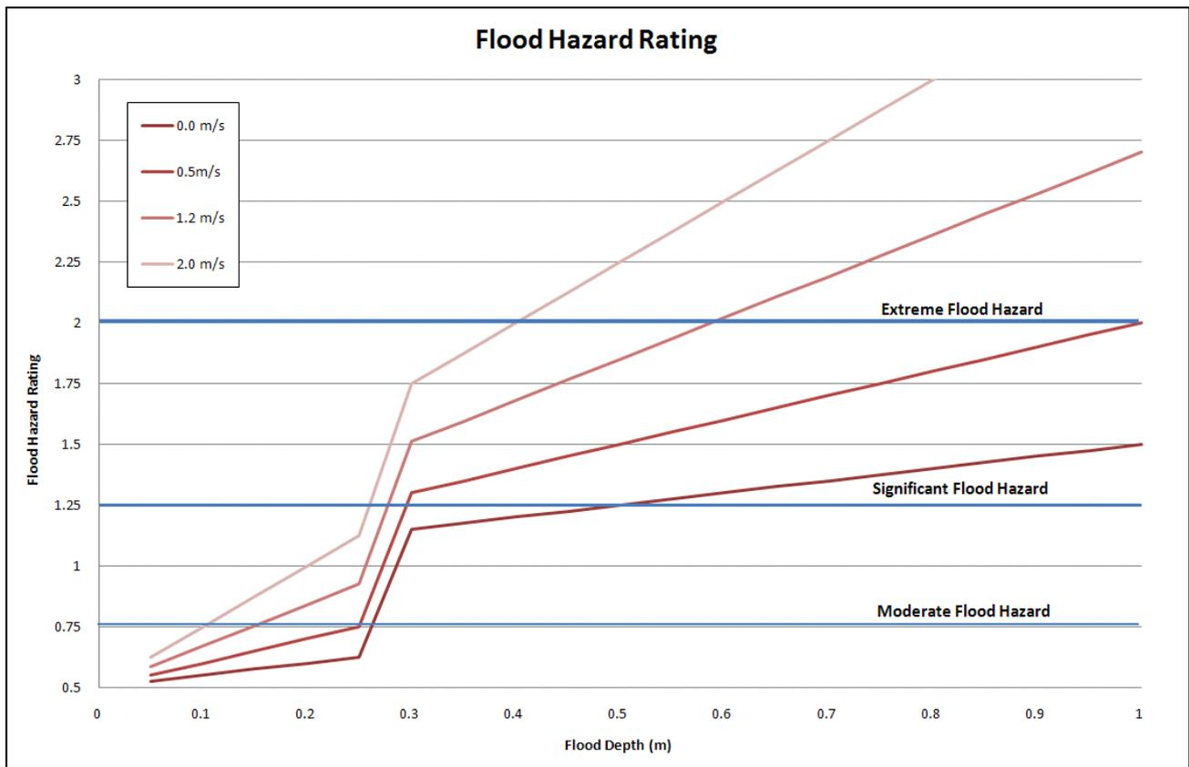
**Figure 5-4: Flood Hazard Rating details**
