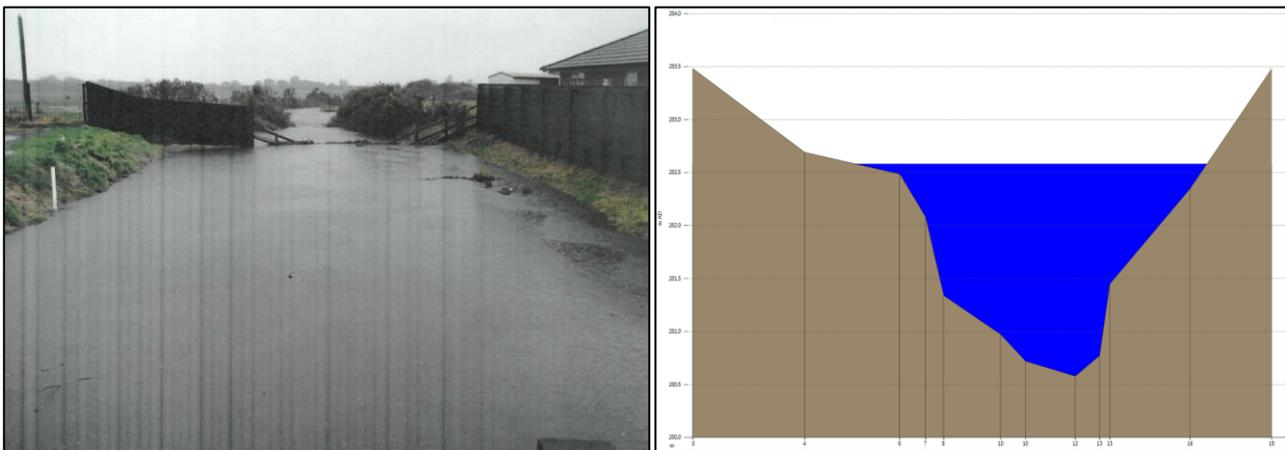
Figure 4-3: Comparison of Stream Levels downstream of Carroll Place
