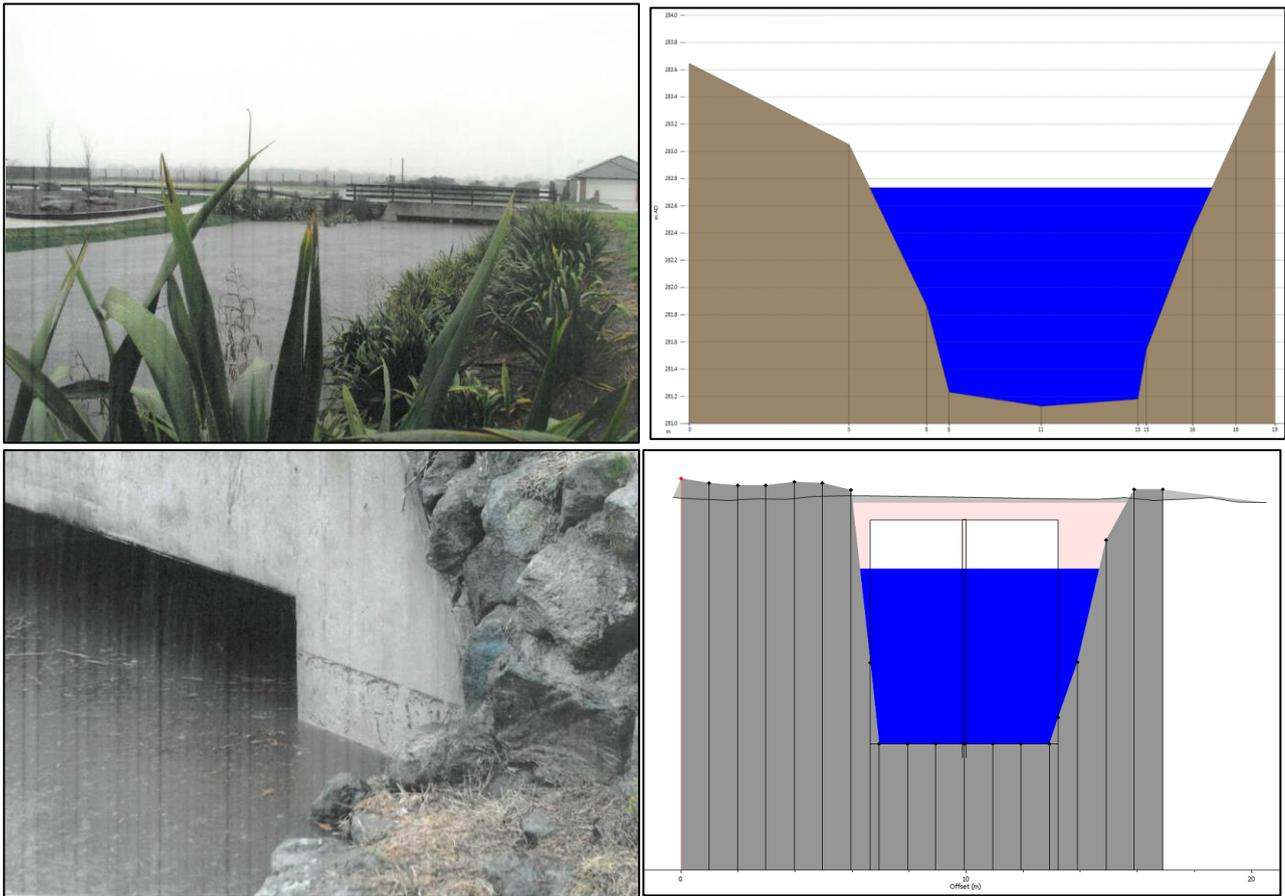
Figure 4-2: Comparison of Stream Levels at the Carroll Place Culvert
