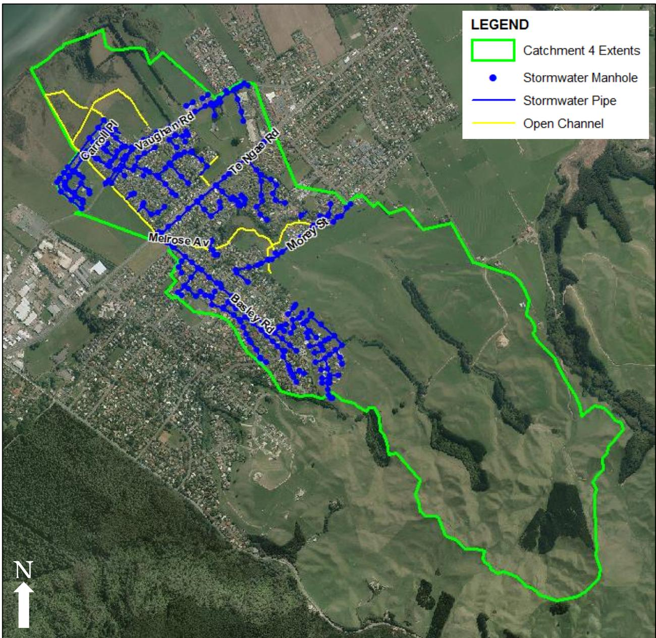
Figure 2-4: Catchment 4 Stormwater Network
