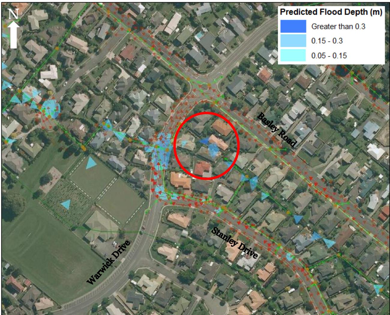
Figure 5-3: Predicted Ponding at Warwick Drive (10% AEP)
