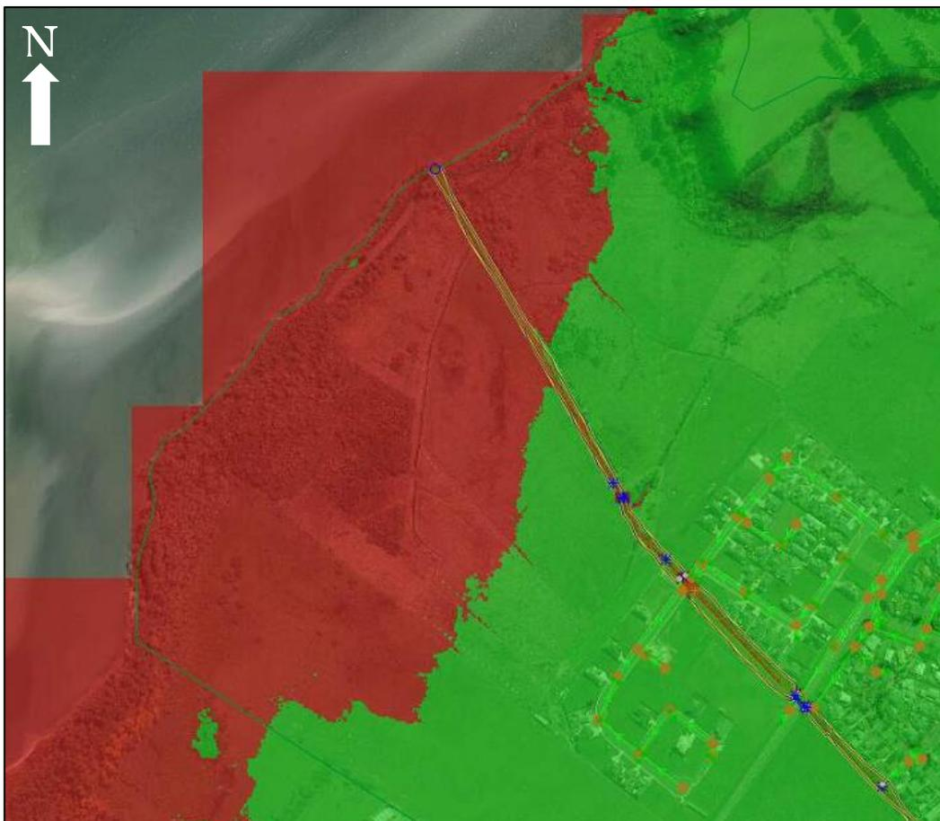
Figure 3-3: Extent of Catchment 4 lower than the 1 in 50 Year ARI Level
