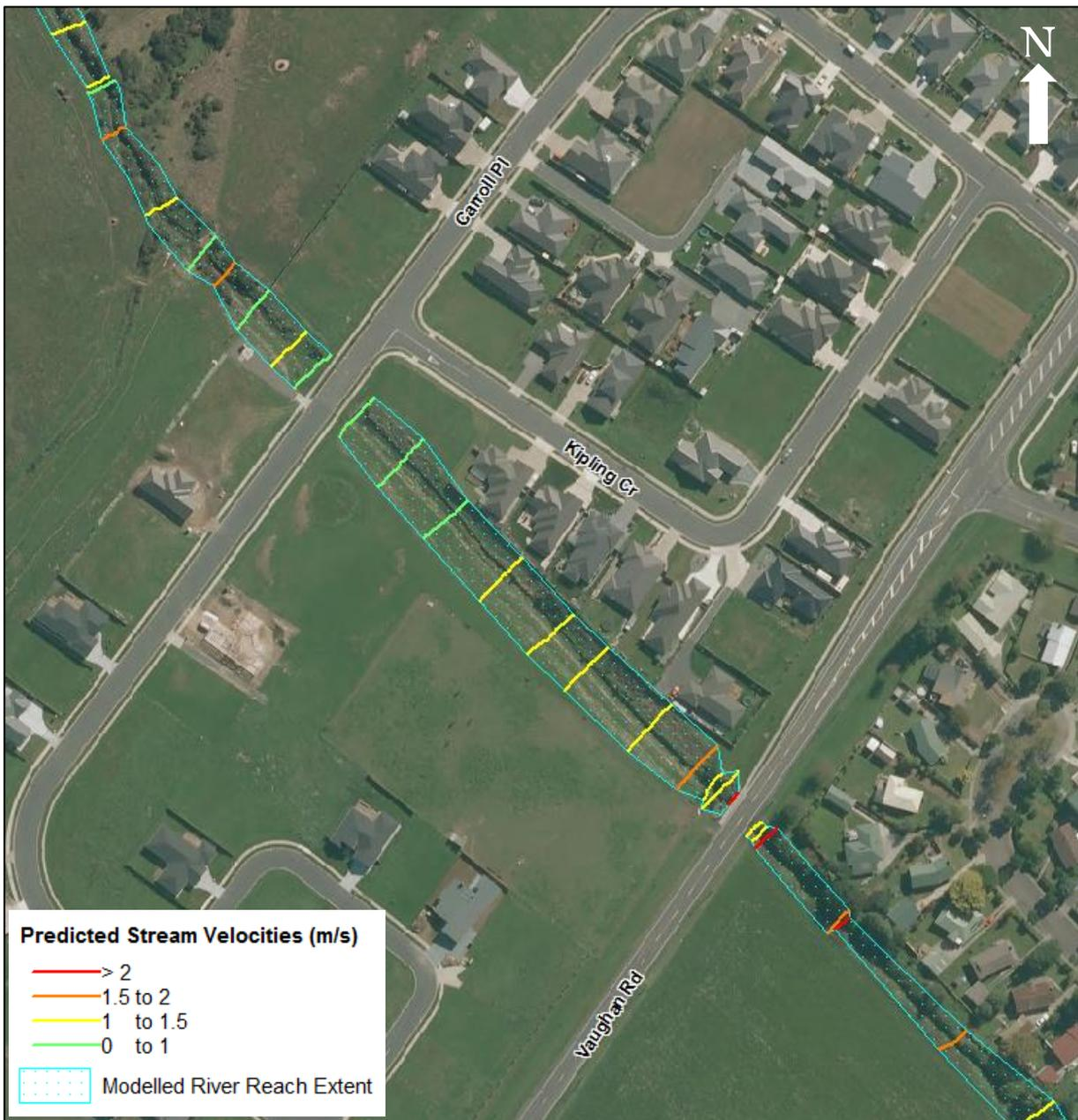
Figure 5-5: Predicted Velocities in Modelled Stream
