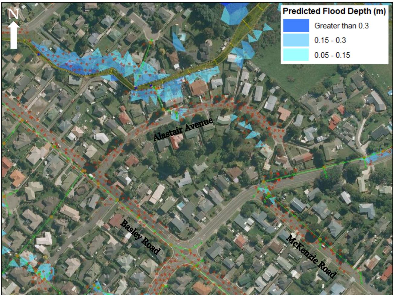
Figure 5-2: Predicted Ponding at Melrose Avenue (10% AEP)
