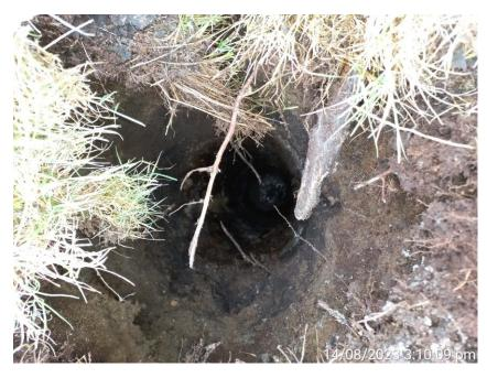
Initial hole picture. Water present in bottom of hole. 350mm of wet muddy soil retrieved from bottom of hole during drilling operations.
