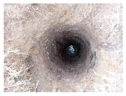
Initial hole picture. Water present in bottom of hole. 250mm of wet muddy soil retrieved from bottom of hole during drilling operation.
