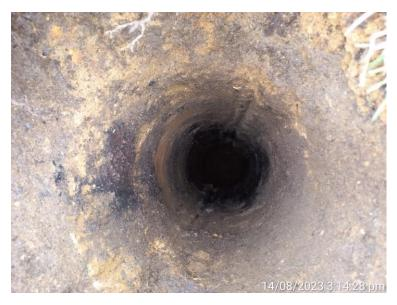
Initial hole picture. No sign of water egress or wet soils.
