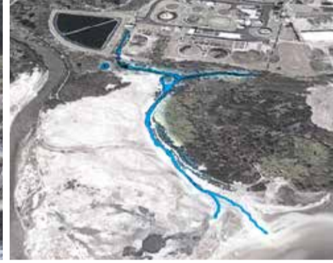
The blue line in this aerial photo shows where the recovered water would flow from the Wastewater Treatment Plant at the top of the image.
