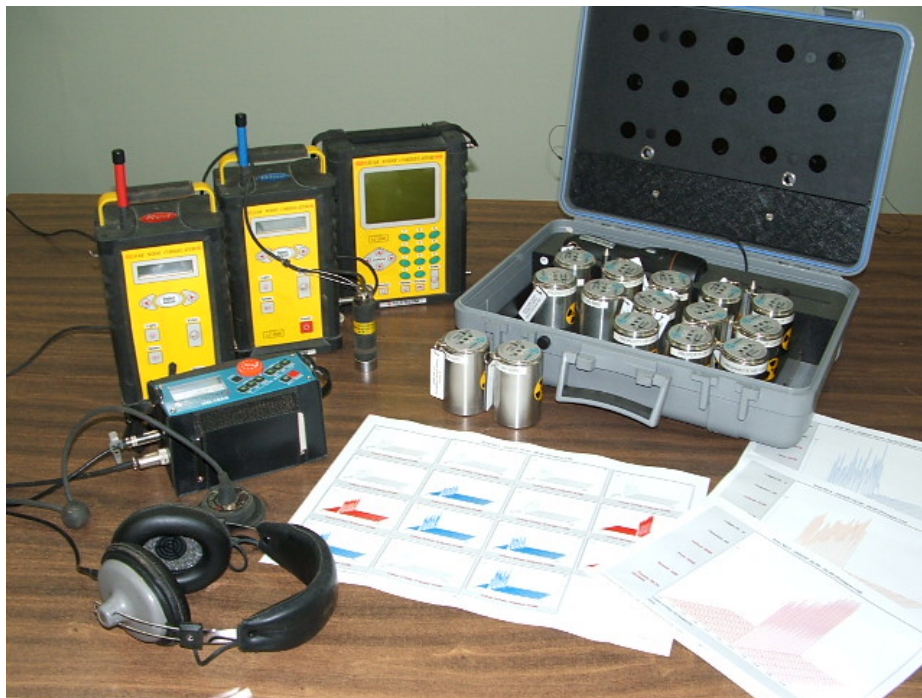
Leak detection equipment – noise loggers which detect water leaks at night time, a leak correlator which is used to pinpoint exact location of water leaks, and a ground microphone used to confirm size
