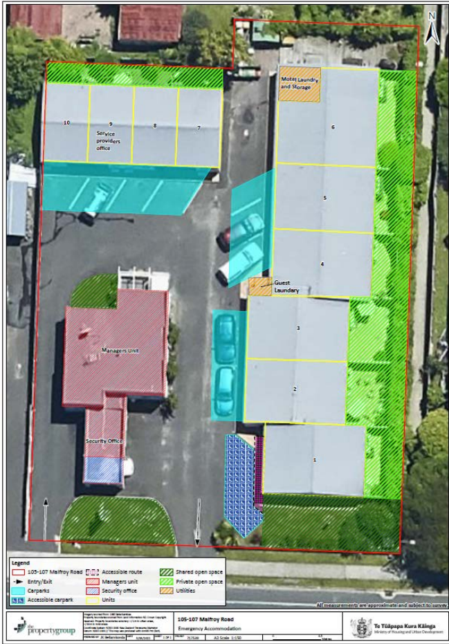
Figure 3: Site plan showing number of units, carparking, managers unit, shared and private open space.
