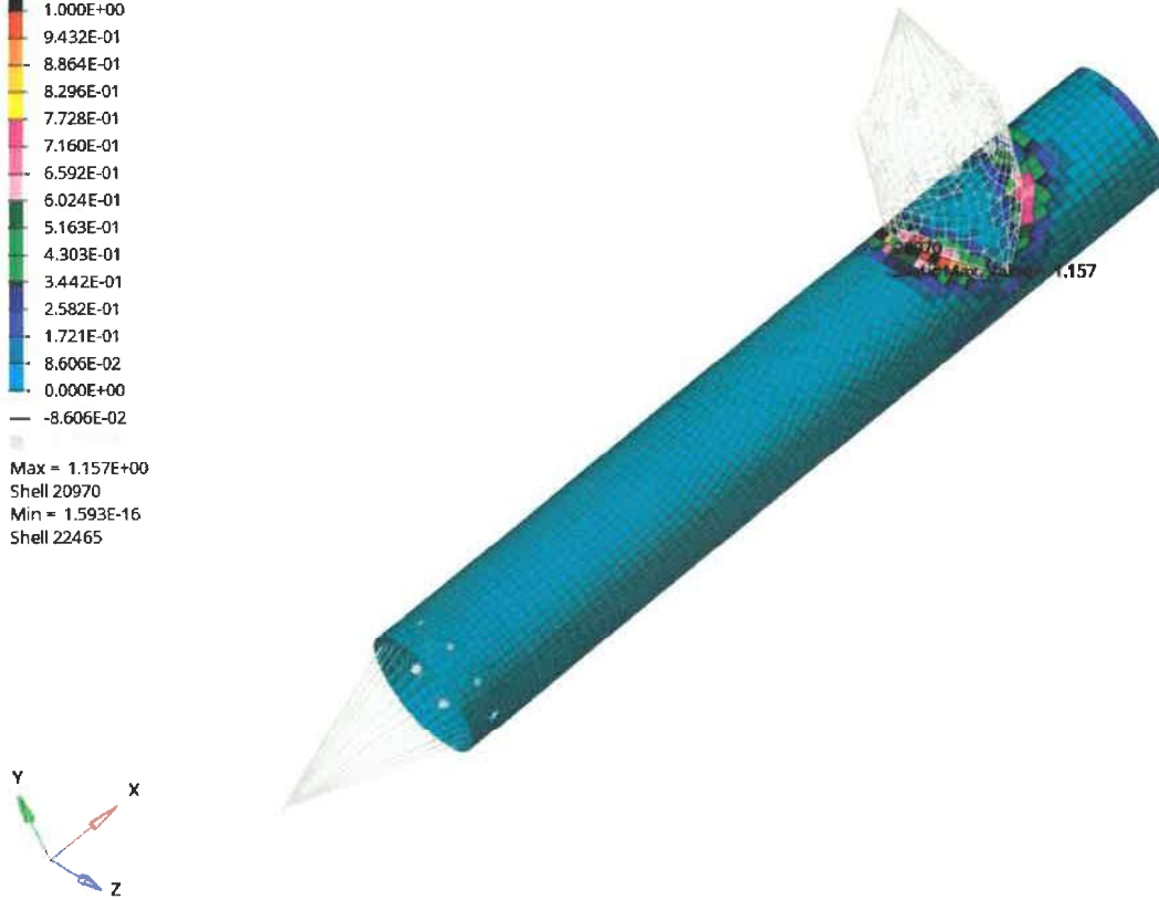
Figure 5. Test model bond failure index
