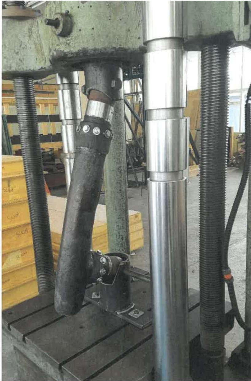
Figure 6. tube assembly installed in mechanical testing rig
