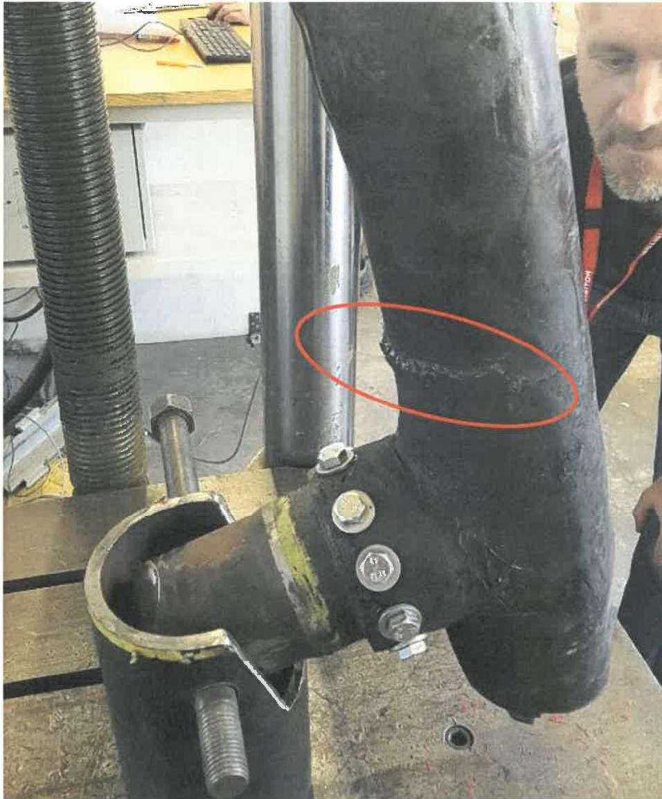
Figure 10. Post max load test, showing compressive failure in inner tube
