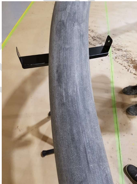
Figure 1. Example of outer tube final e-glass sock layer during manufacture
