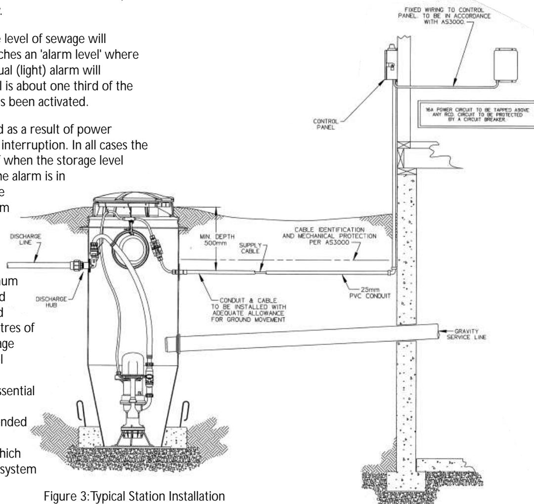
Figure 3: Typical Station Installation
