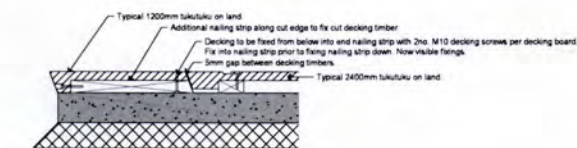
5 Typical 1200mm Tukutuku Bridge to Larger Tukutuku Flush Transition- Detail Scale: 1:10@ A1 | 1:20@A3
