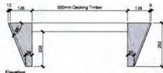
2 1200mm Tukutuku Bridge - Decking Type S Scale: 1:5 @ A1 | 1:10 @A3
