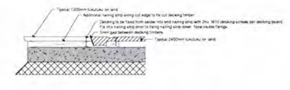
5 Typical 1200mm Tukutuku Bridge to Larger Tukutuku Flush Transition - Detail Scale: 1:100 A1 | 1:200 A2
