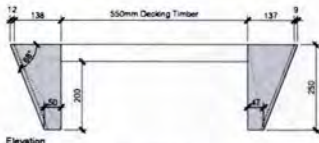
1 1200mm Tukutuku Bridge - Decking Type R Scale: 1:5 @ A1 | 1:10 @A3
