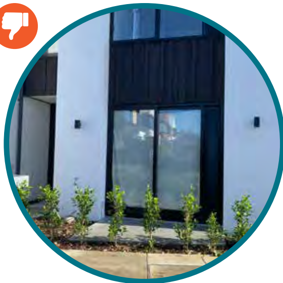
Terraced House, Hobsonville. A full-height window to the street with minimal landscaping and no fencing compromises privacy resulting in drawn blinds and limited potential to contribute to passive surveillance.
